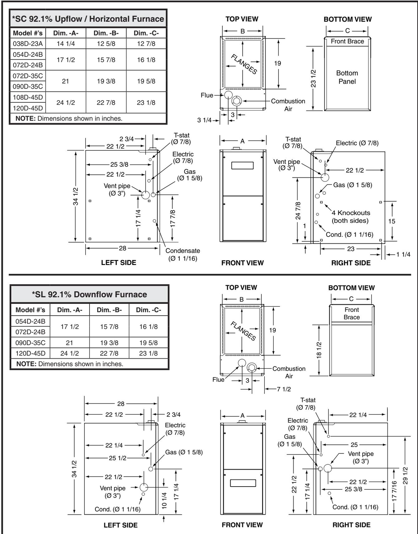
**Figure 31. Furnace Dimensions**
