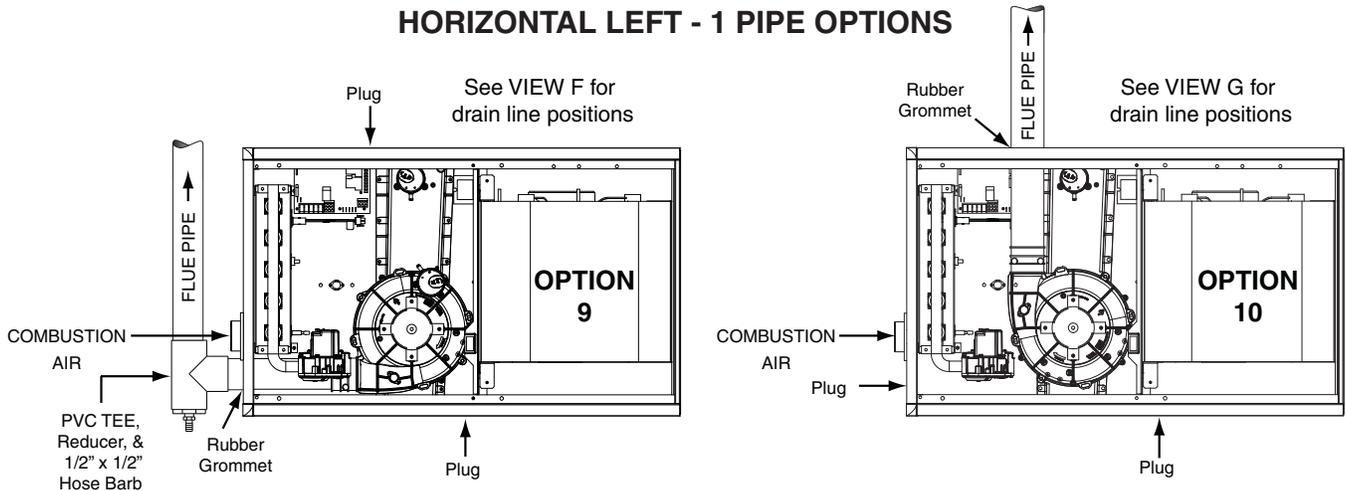
**Figure 35. Horizontal Options - 1 Pipe Furnaces**
