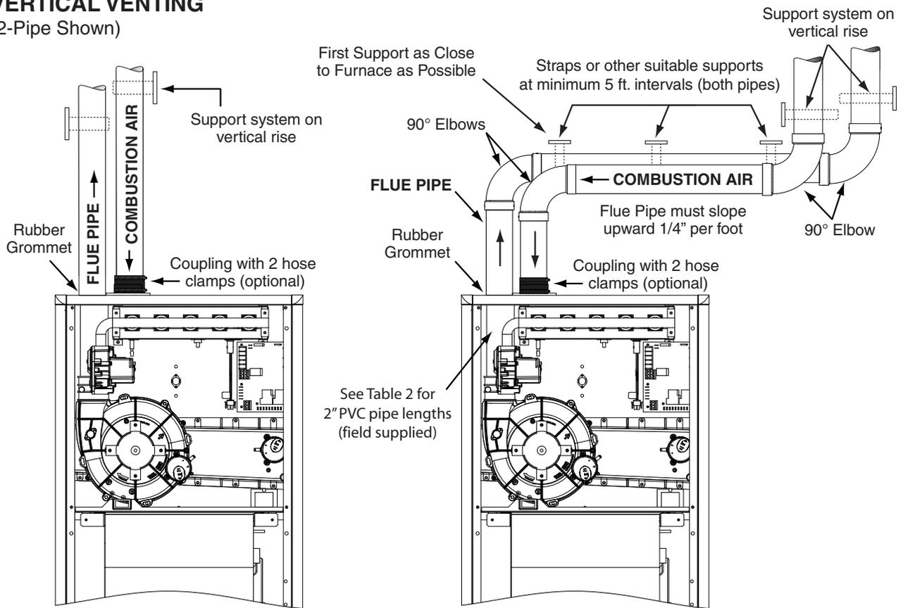
Figure 33. Horizontal & Vertical Venting
