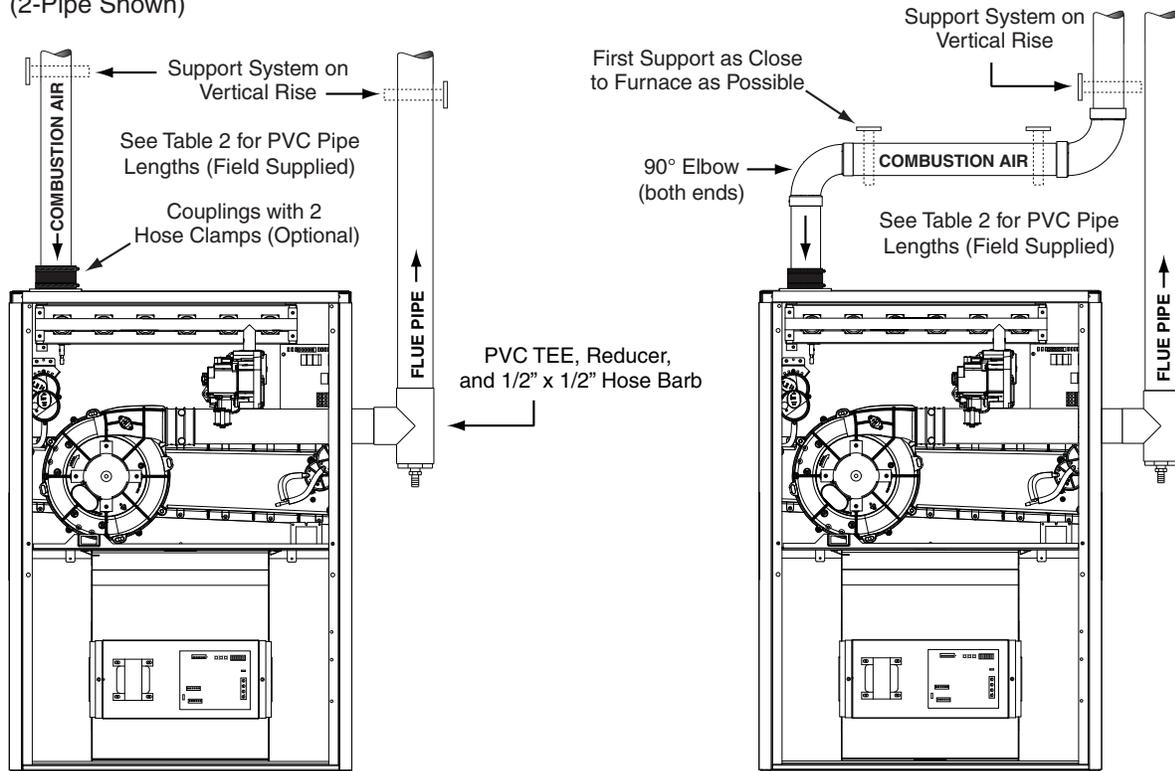
**Figure 37. Horizontal and Vertical Venting**
