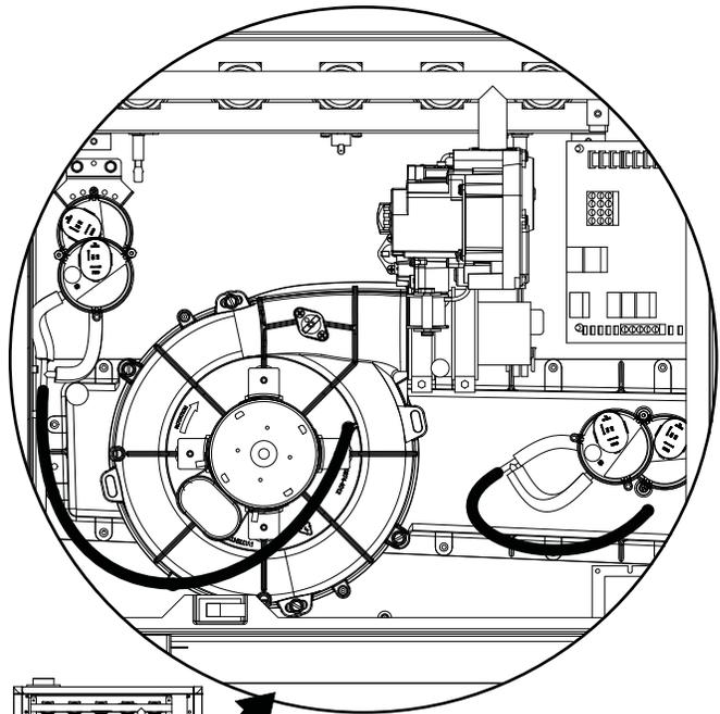
**Figure 15. Pressure Switch Tubing for \*TC Upflow / Horizontal Furnaces**
