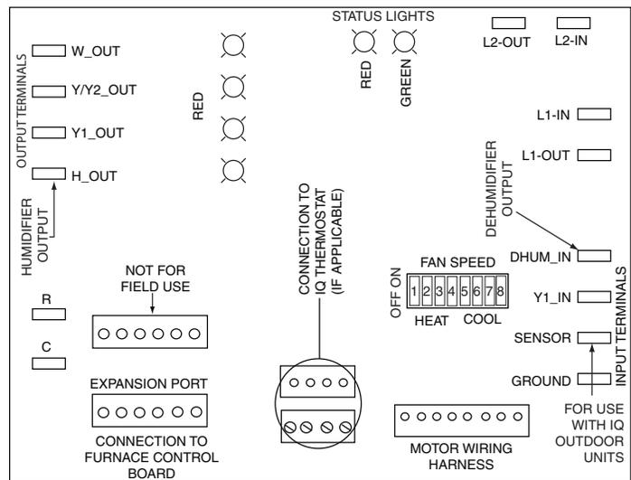
**Figure 31. Two-Stage Variable Speed Motor Control Board**
