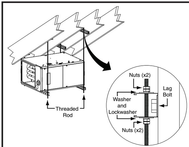
Figure 13. \*TC Horizontally Suspended in an Attic
