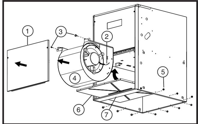
Figure 20. Bottom Panel Removal
