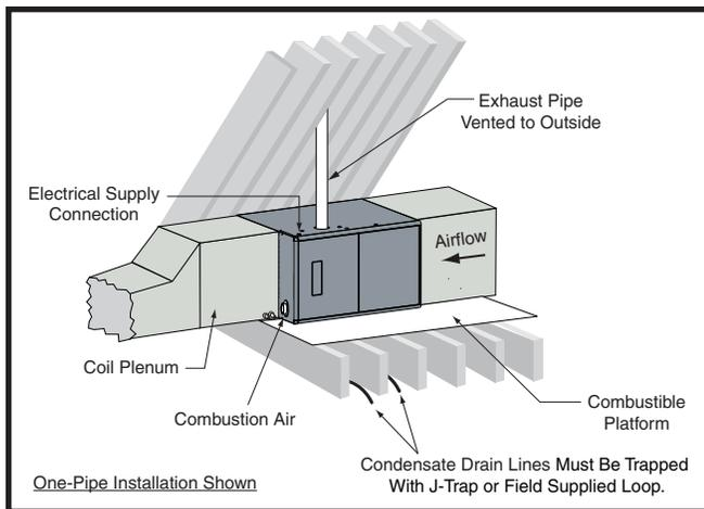
Figure 12. \*TC Horizontally Installed on a Platform
