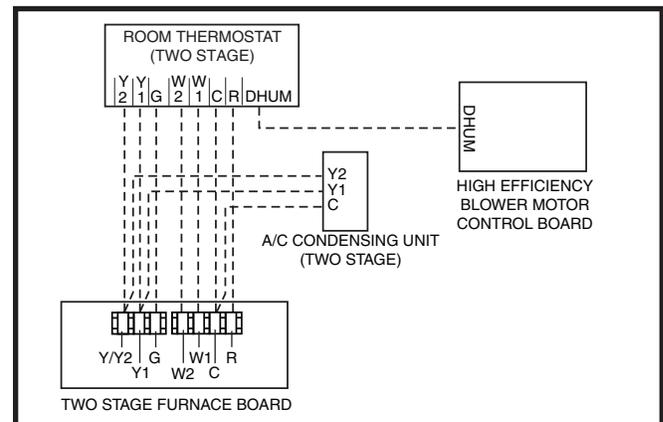
Figure 26. Wiring Configuration 3
