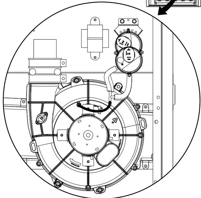
**Figure 16. Pressure Switch Tubing for Downflow Furnaces**
