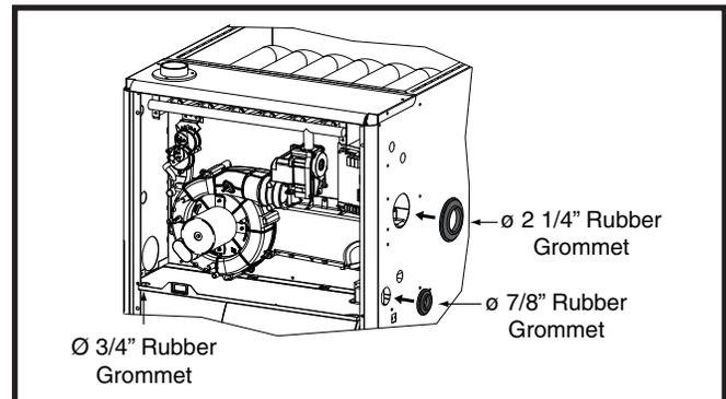
Figure 18. Rubber Grommets
