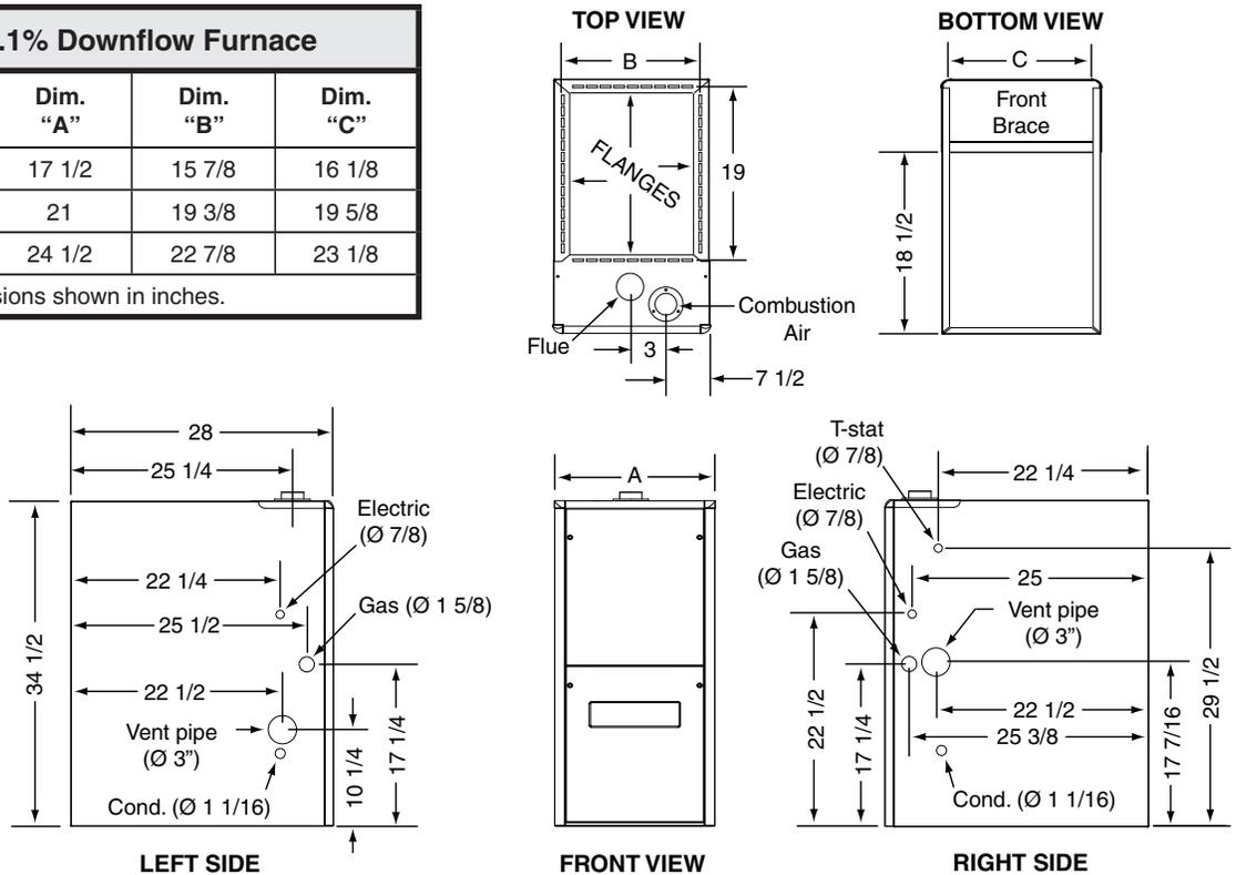
**Figure 29. Furnace Dimensions**
