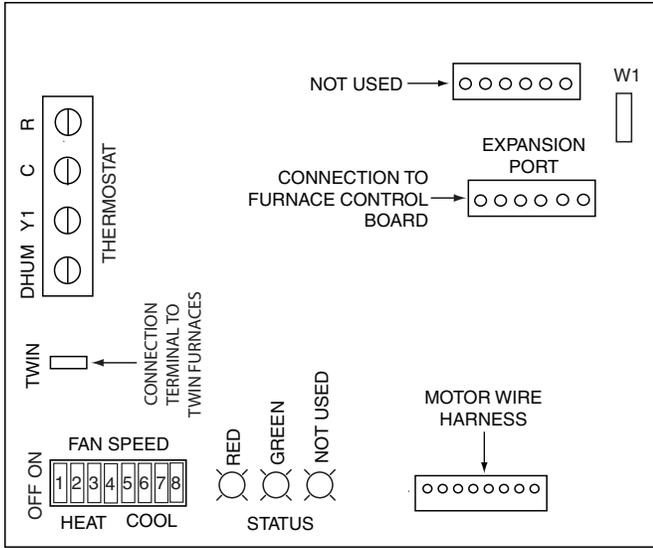
**Figure 30. Two-Stage Fixed Speed Motor Control Board**
