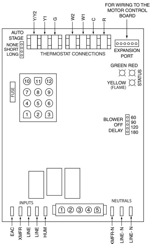
**Figure 32. Two-Stage Furnace Control Board**
