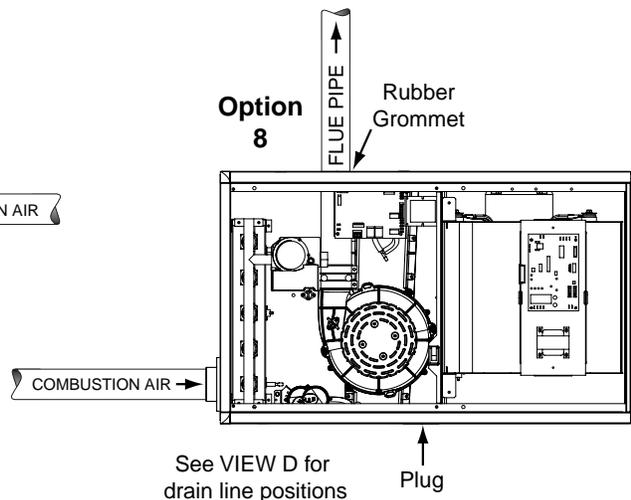
**Figure 27. Vent Pipe & Condensate Options - Horizontal Furnaces**
