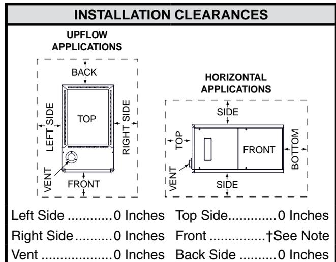
†NOTE: Allow 24 inches minimum clearance for servicing. Recommended clearance is 36 inches.
