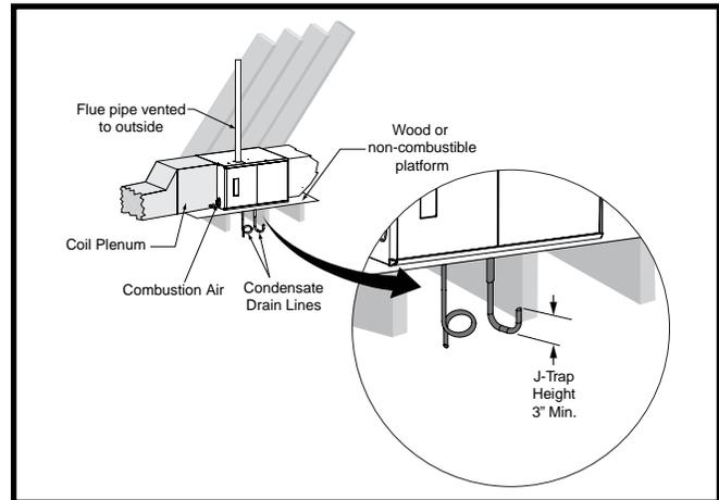
**Figure 11. Horizontal installation on a Platform**
