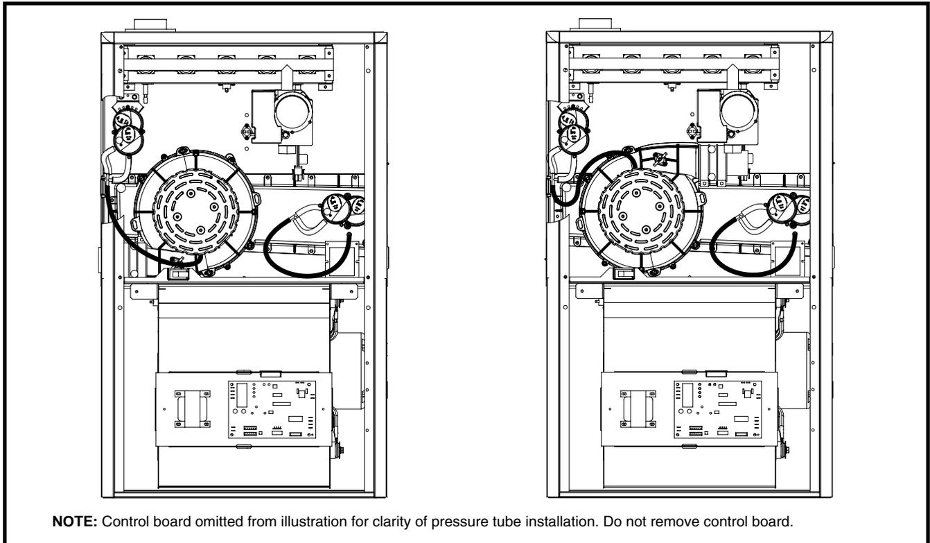
**Figure 17. Pressure Switch Tubing for \*MQ Upflow / Horizontal Furnaces**
