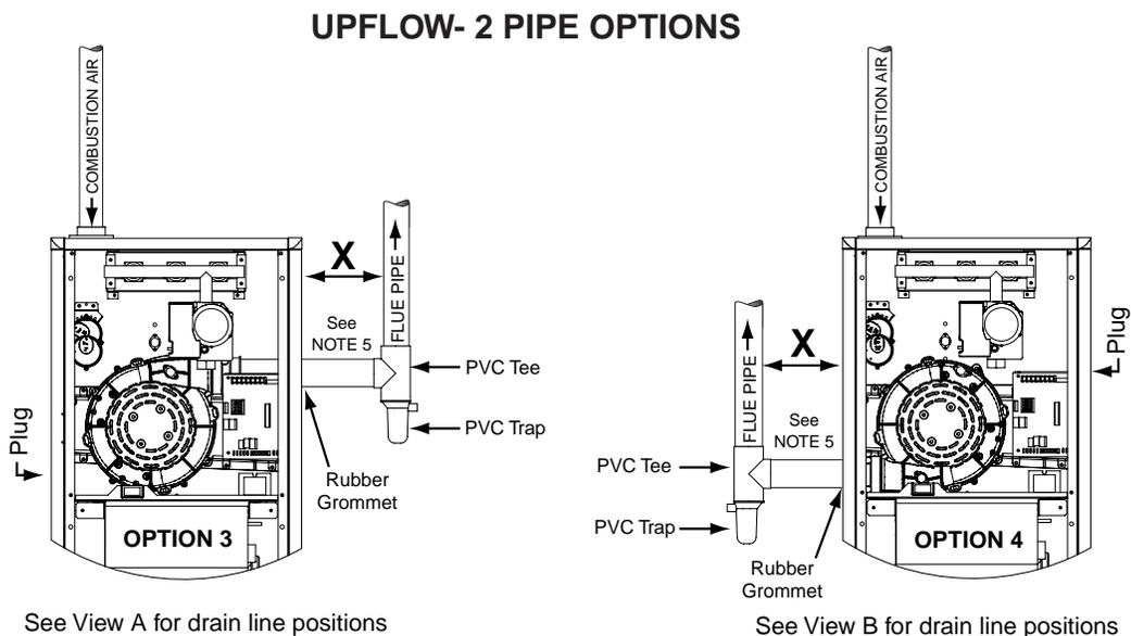
**Figure 26. Vent Pipe & Condensate Options - Upflow Furnaces**
