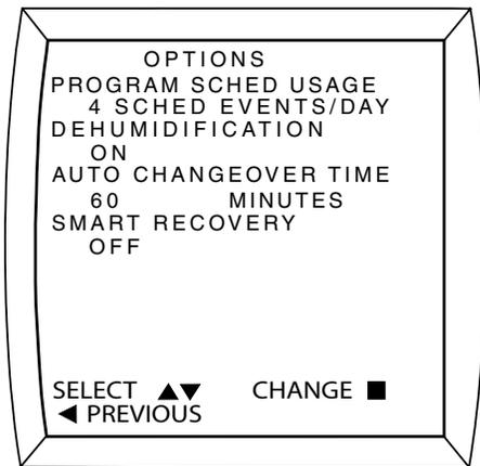
4. Use the ▲ or ▼ key to select the value under AUTO CHANGEOVER TIME, then press the ■ key to allow changing the setting.
