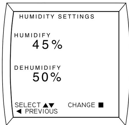
3. Use the ▲ or ▼ key to select the RH setting to change, then press the ■ key to allow changes.
