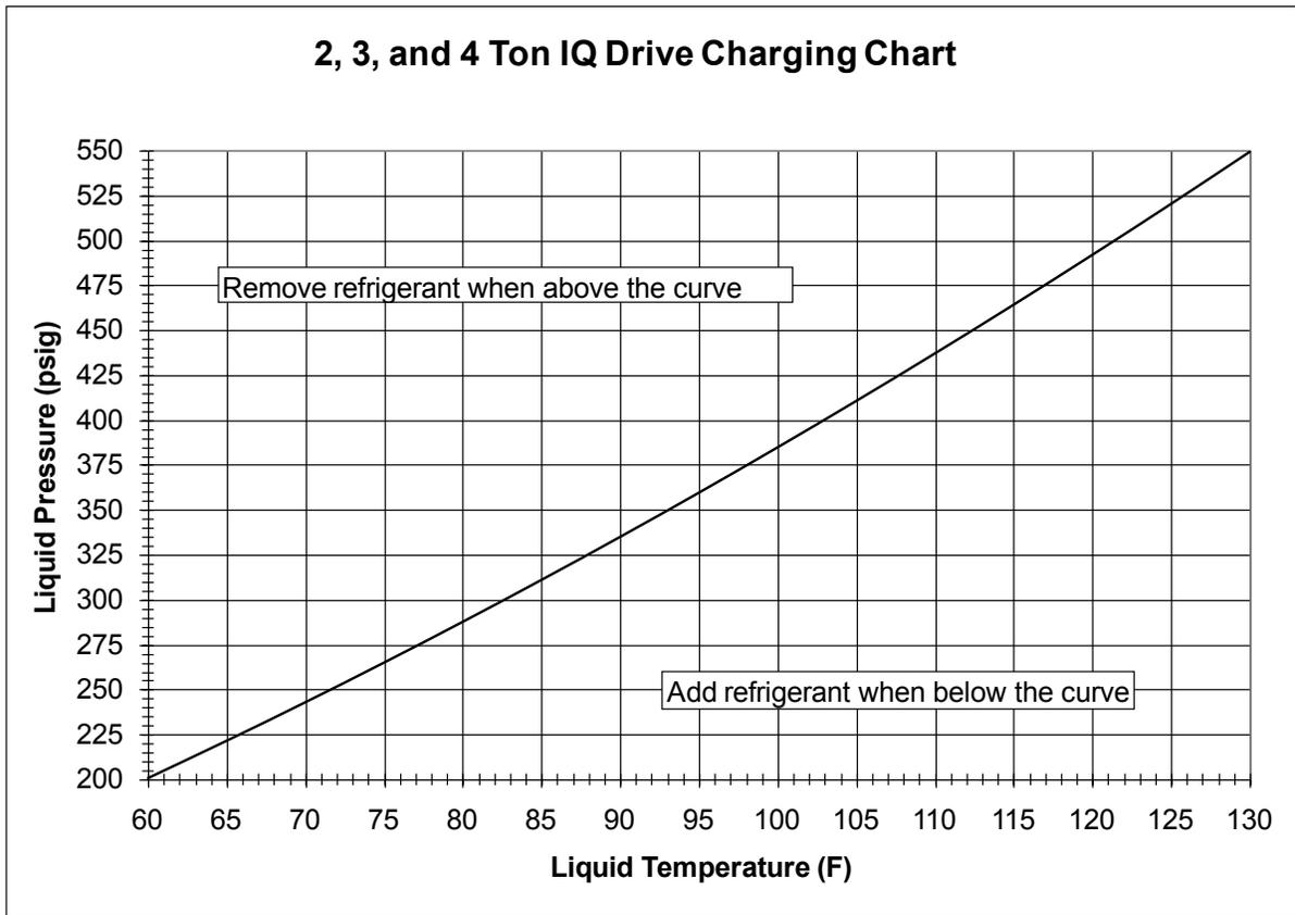
Figure 9. Charging Chart for iQ Drive Air Conditioning
