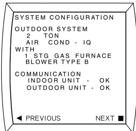
The words under OUTDOOR SYSTEM and WITH describe the system components as automatically detected by the controller. Both entries under COMMUNICATION should show “OK”. If “CHECK” appears, it is an indication that either communication wiring is incomplete or incorrect, or the outdoor
