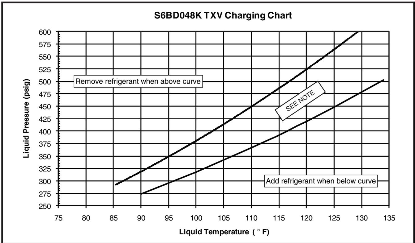
Figure 11. Charging Chart for 4 Ton Units
