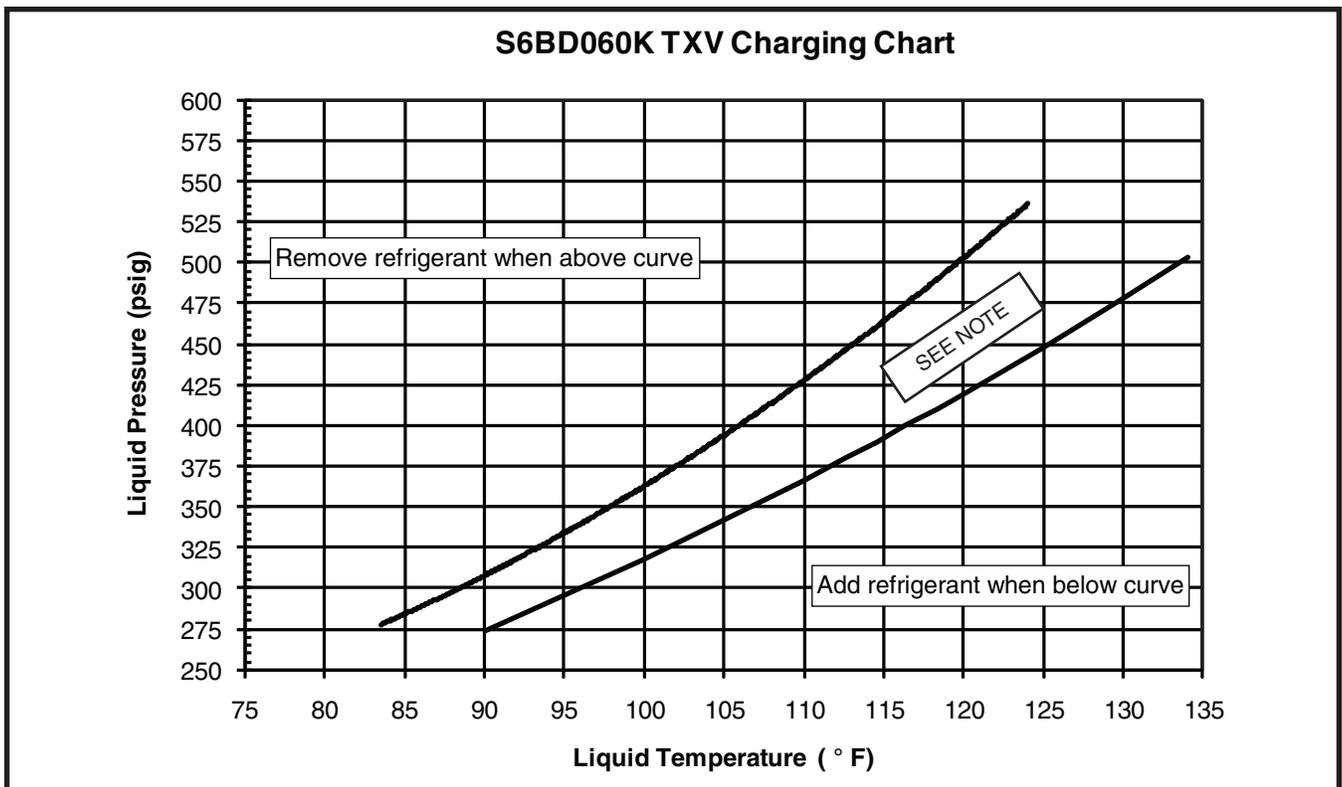
Figure 12. Charging Chart for 5 Ton Units
