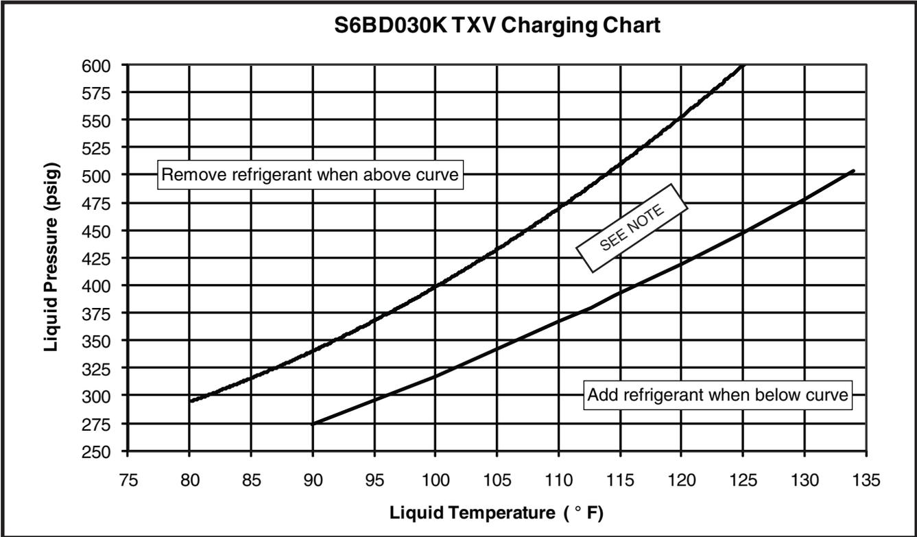
Figure 8. Charging Chart for 2.5 Ton Units
