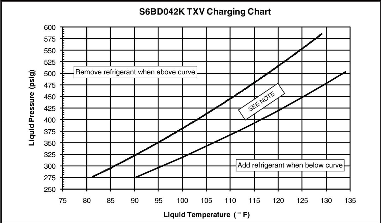
Figure 10. Charging Chart for 3.5 Ton Units
