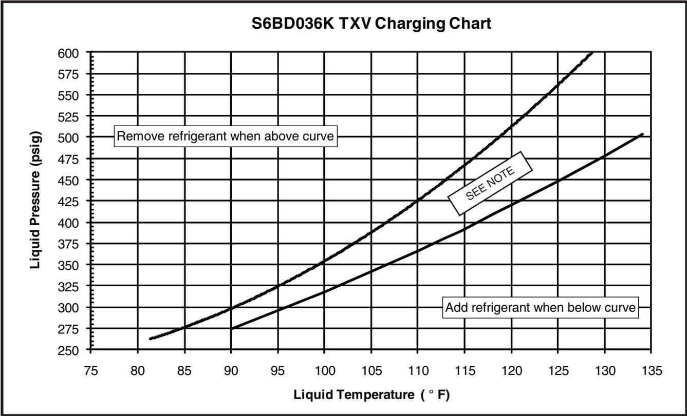
Figure 9. Charging Chart for 3 Ton Units
