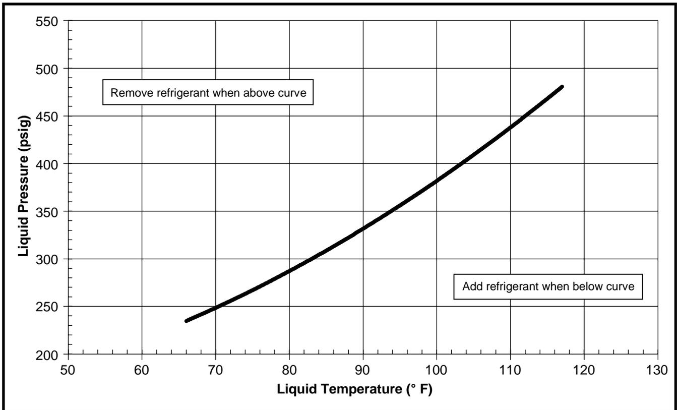
Figure 20. Charging Chart for 3 Ton Units
