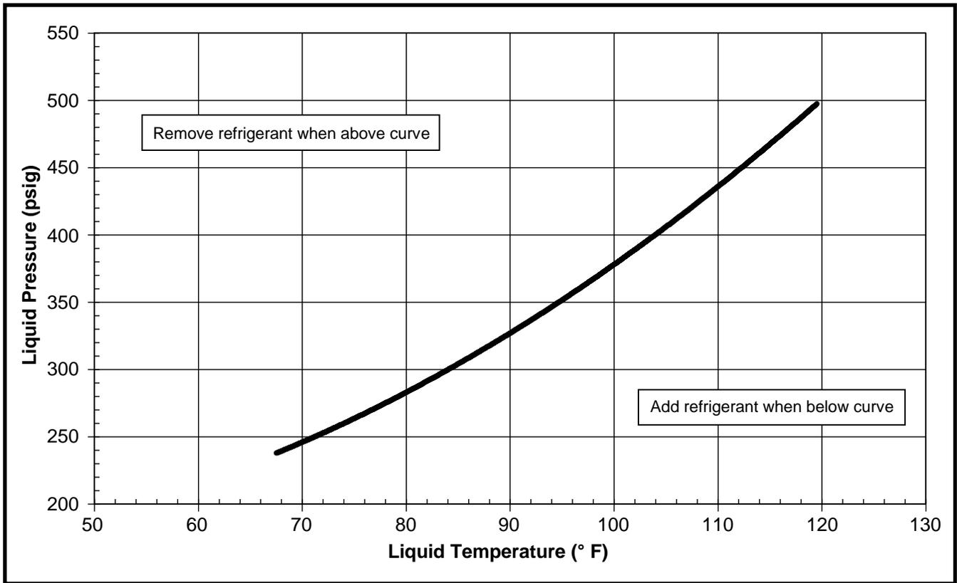
Figure 21. Charging Chart for 4 Ton Units
