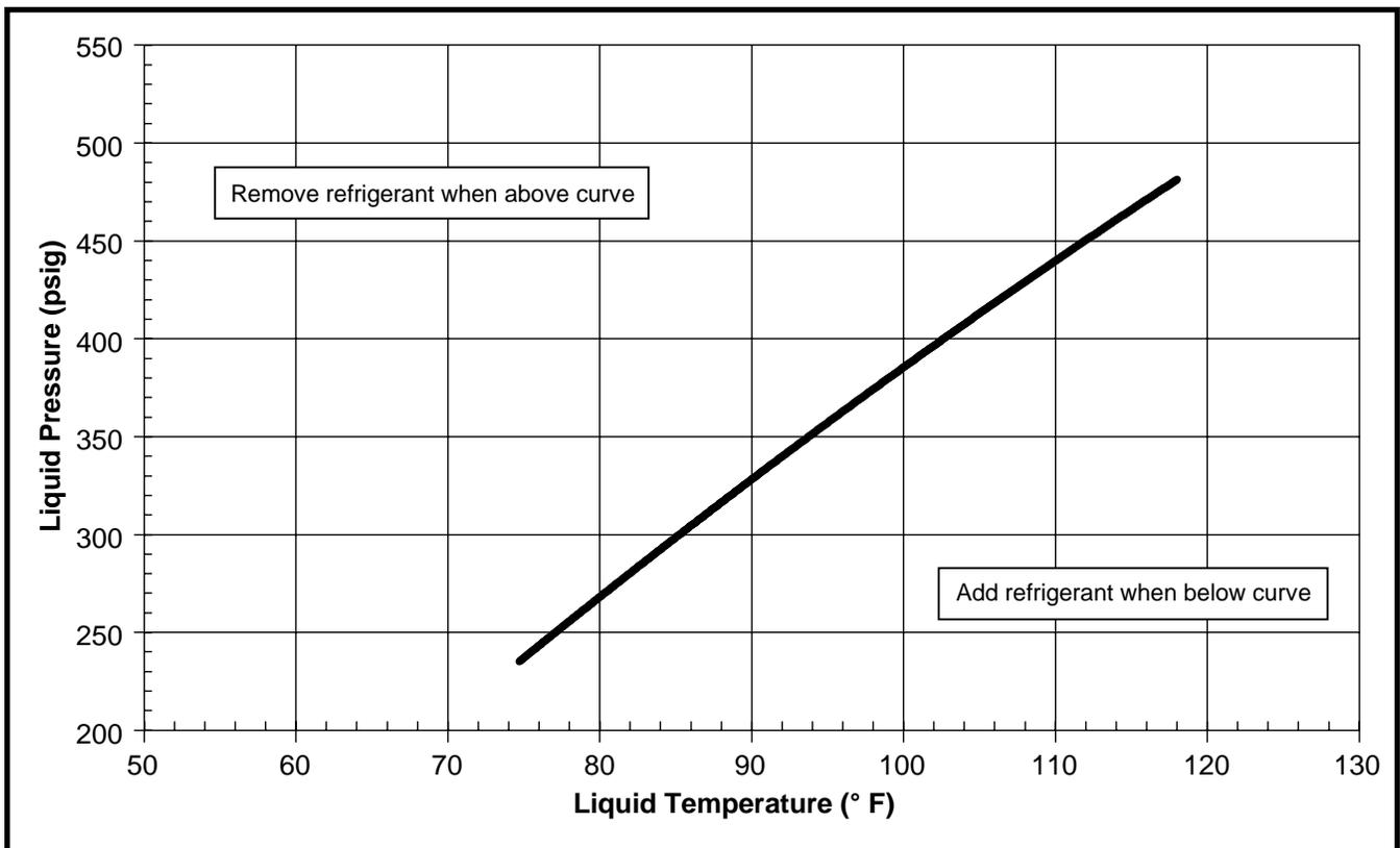
Figure 22. Charging Chart for 5 Ton Units
