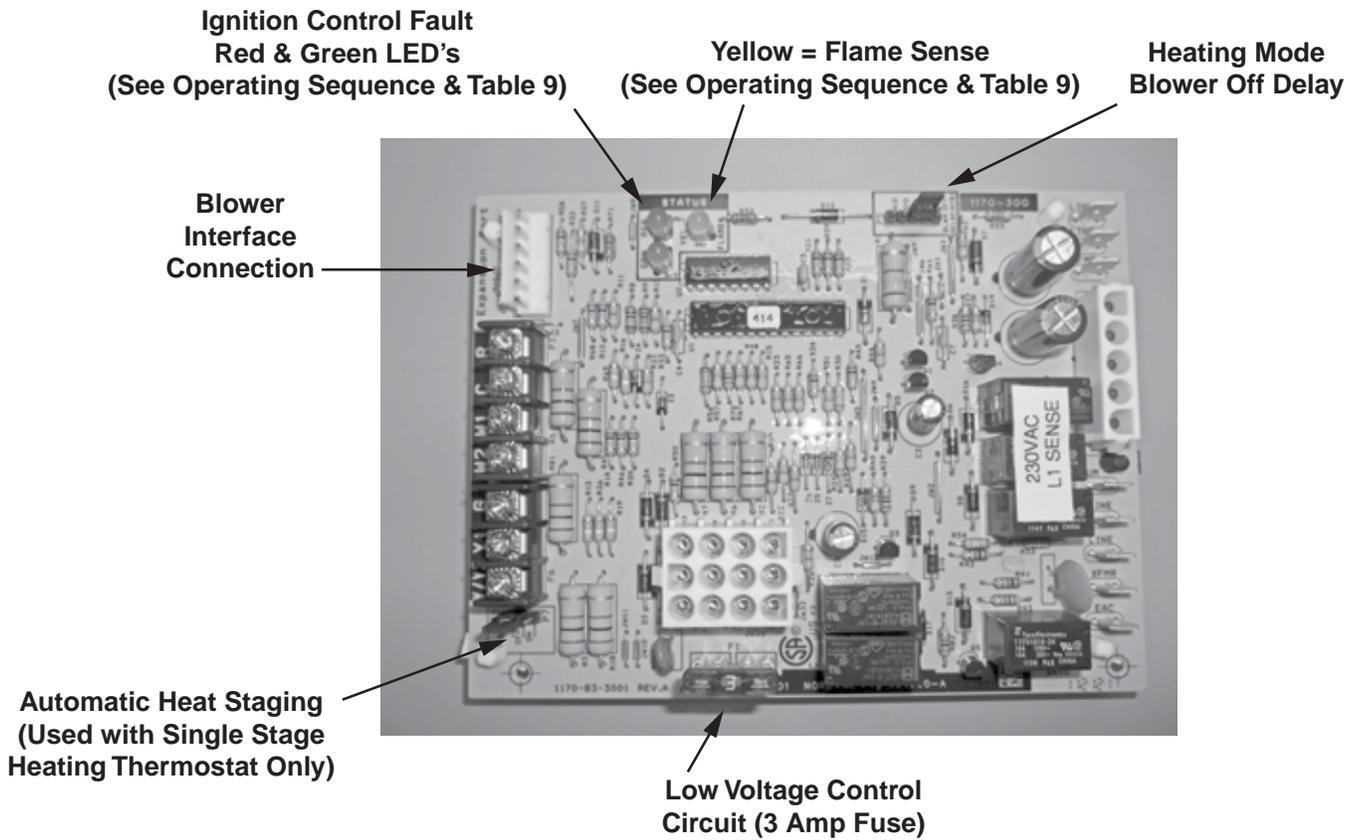
**Figure 12. Two-Stage, Hot Surface Ignition & Blower Control Board**
