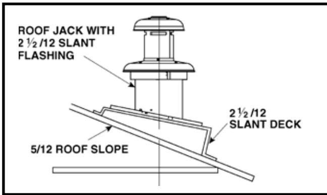
Figure 18. Example of 2½ / 12 Slant Jack with Flashing
