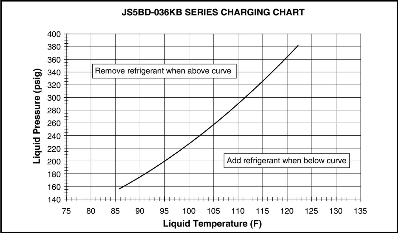
Figure 8. Charging Chart for 3 Ton Units (with Microchannel Coil)
