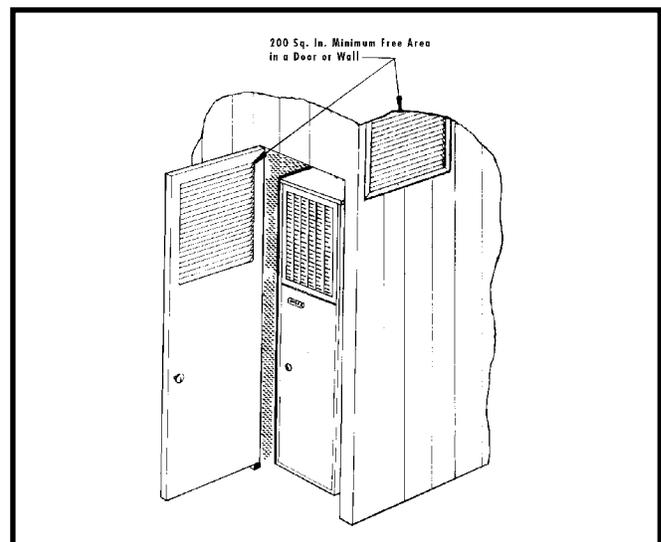
**Figure 6. Closet Installation**
