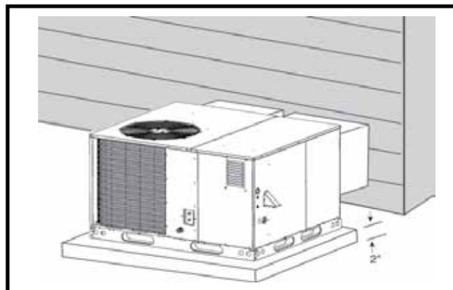
**Figure 3. Ground Level Installation**
