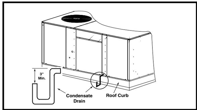
**Figure 2. Condensate Drain**
