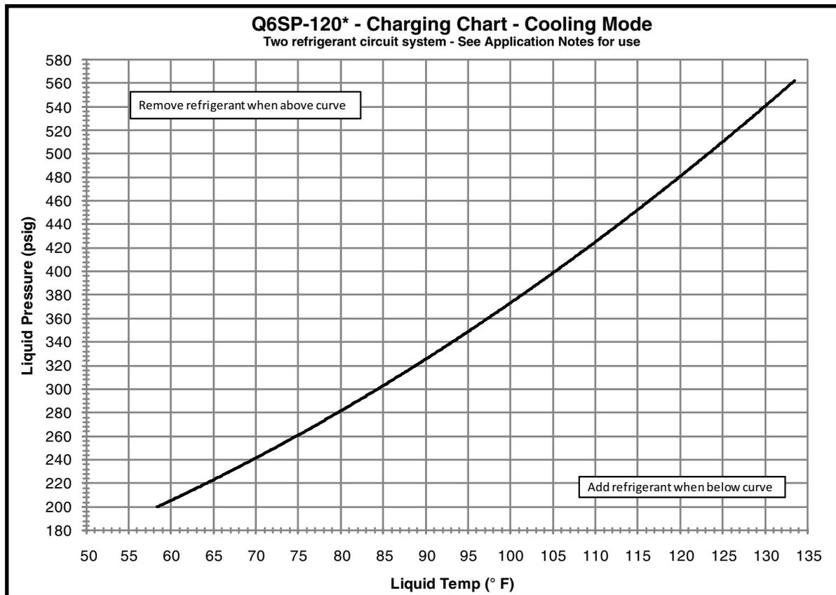
**Figure 14. Charging Chart for 10 Ton Units**
