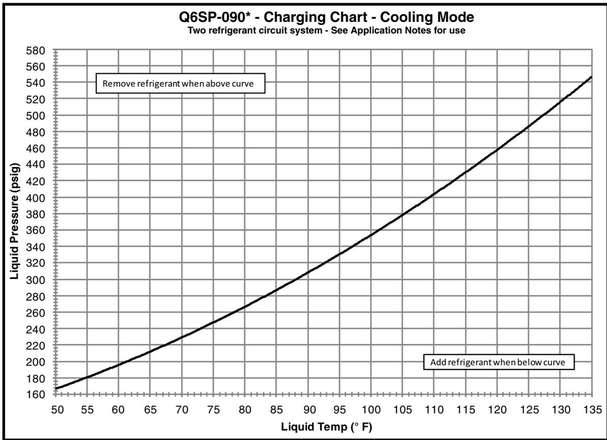
**Figure 13. Charging Chart for 7 1/2 Ton Units**
