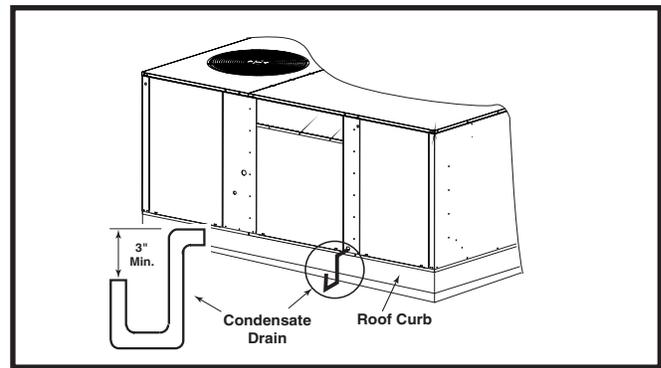
**Figure 2. Condensate Drain**
