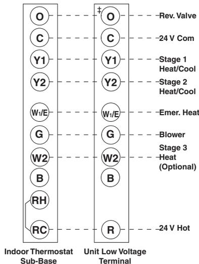
± "O" - Energized when thermostat system is in "Cool" Mode.
