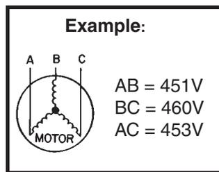
2. Determine the average voltage in the power supply.
