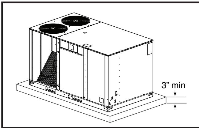
Figure 7. Concrete Pad
