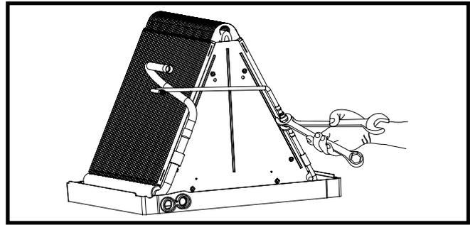
Figure 6. Loosening of Nut & Distributor Body
