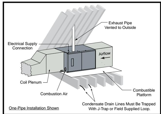
Figure 11. \*TC Horizontally Installed on a Platform
