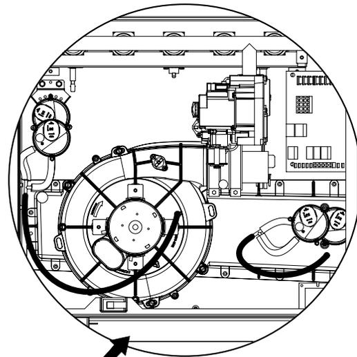
**Figure 14. Pressure Switch Tubing for \*TC Upflow / Horizontal Furnaces**
