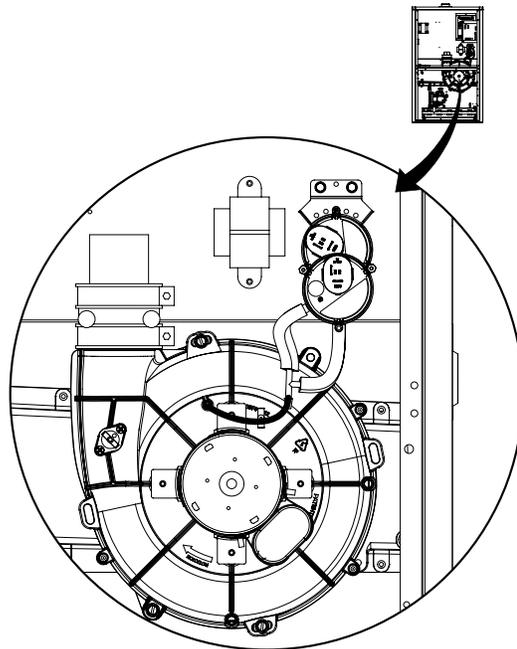
**Figure 15. Pressure Switch Tubing for \*TL Downflow Furnaces**
