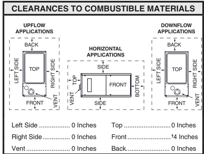
†Allow 24 in. minimum clearance for servicing. Recommended clearance is 36 in.
