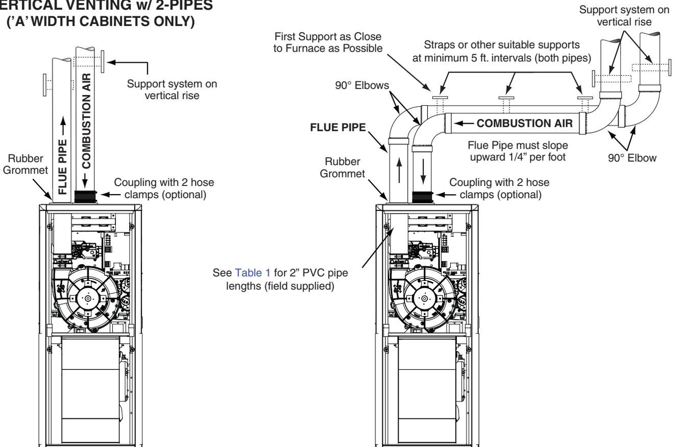
**Figure 36. Horizontal & Vertical Venting (A Width Cabinets)**
