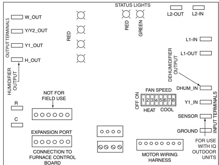
**Figure 30. Two-Stage Variable Speed Motor Control Board**
