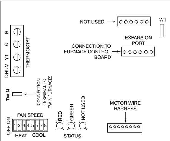
**Figure 29. Two-Stage Fixed Speed Motor Control Board**
