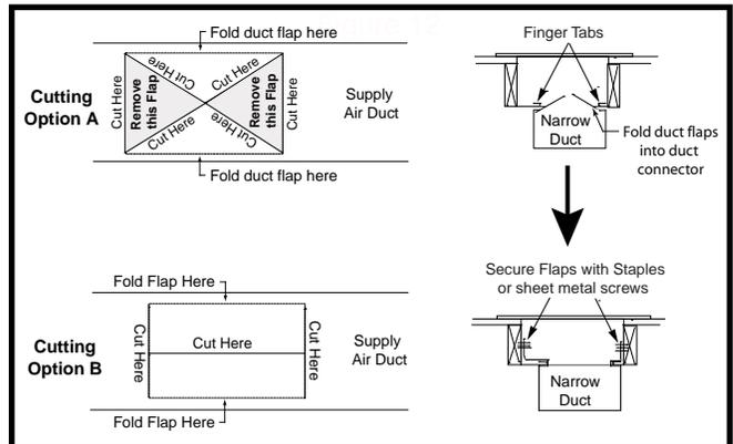
**Figure 12. Narrow Air Ducts - Option 1**
