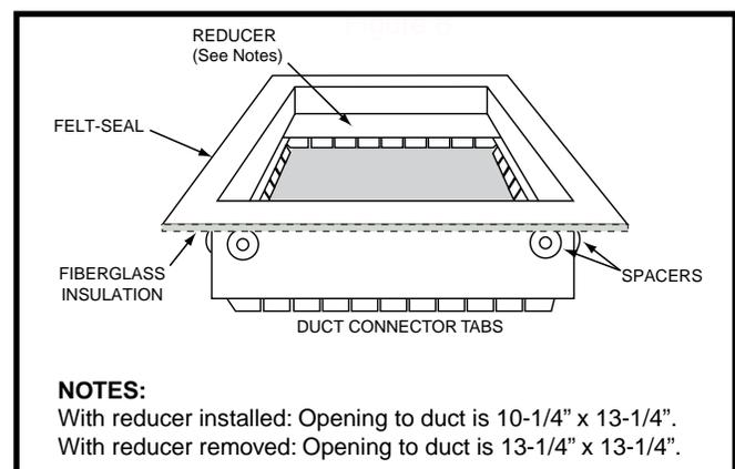
**Figure 8. Duct Connector**
