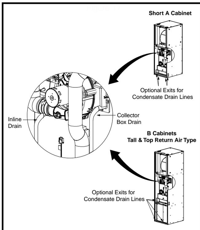
**Figure 17. Condensate Drainage**
