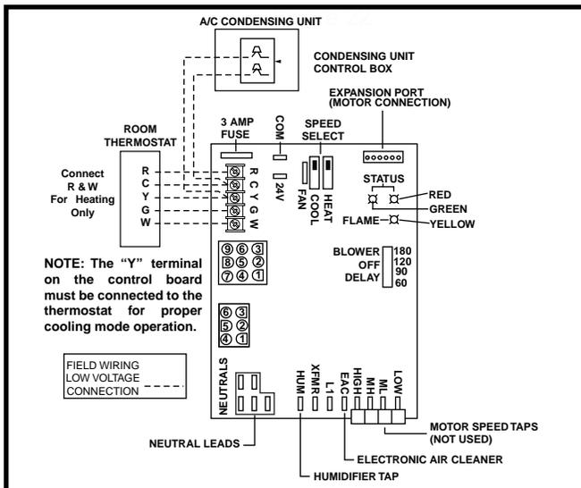
**Figure 22. Low Voltage Field, Four-wire Heating/Cooling Applications**
