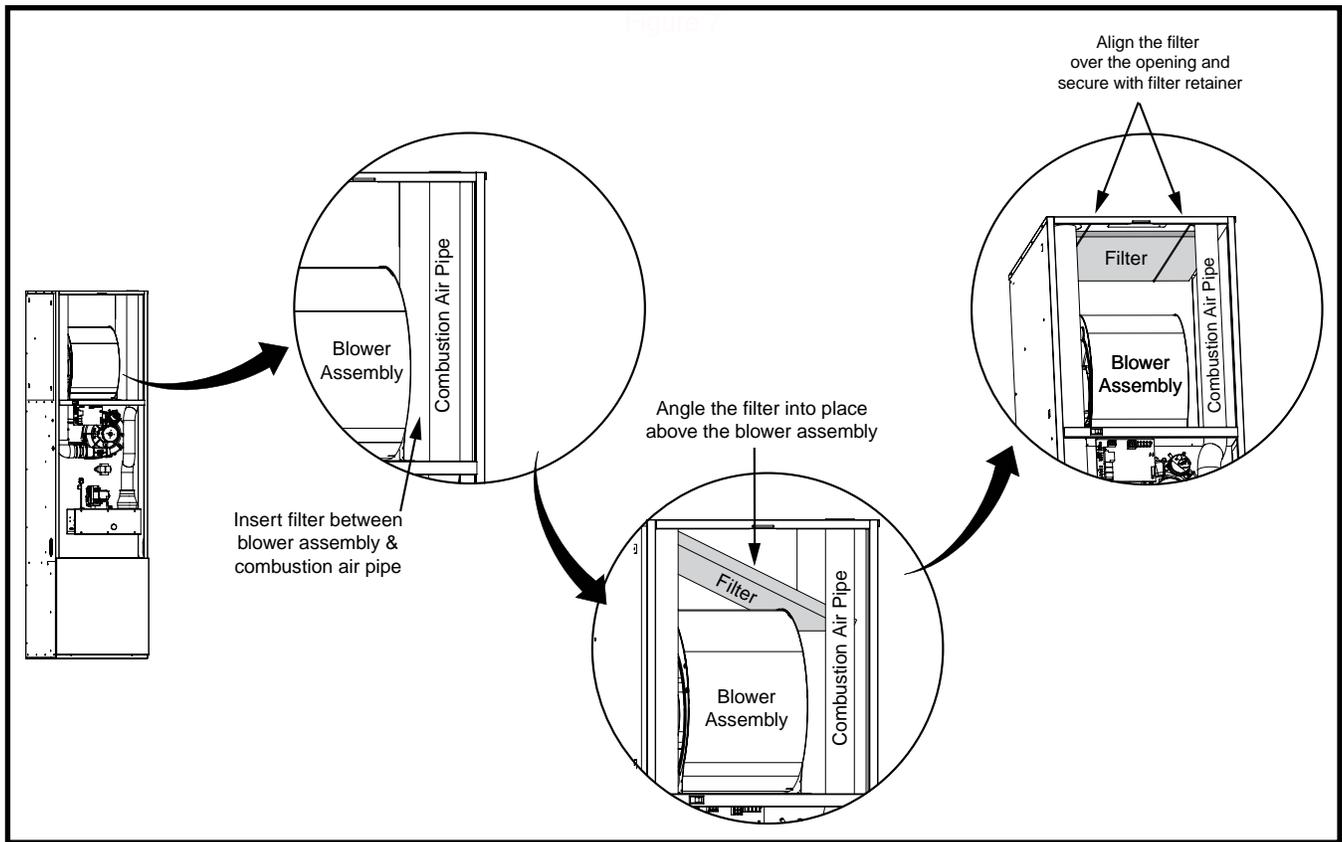
**Figure 7. Filter Installation**
