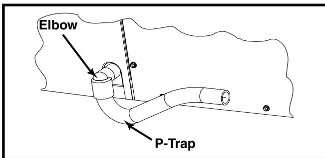
Figure 6. Drain Trap
