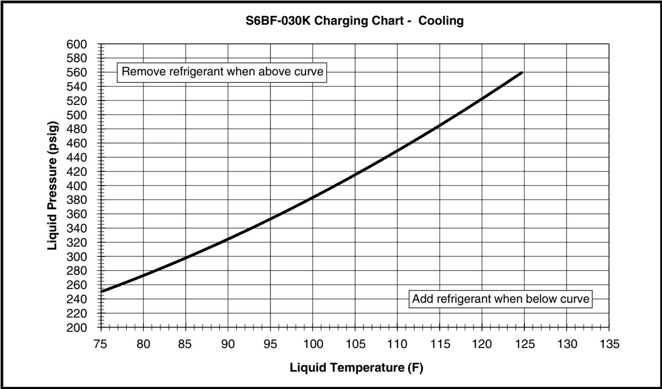
**Figure 3. Charging Chart for 2.5 Ton Units
