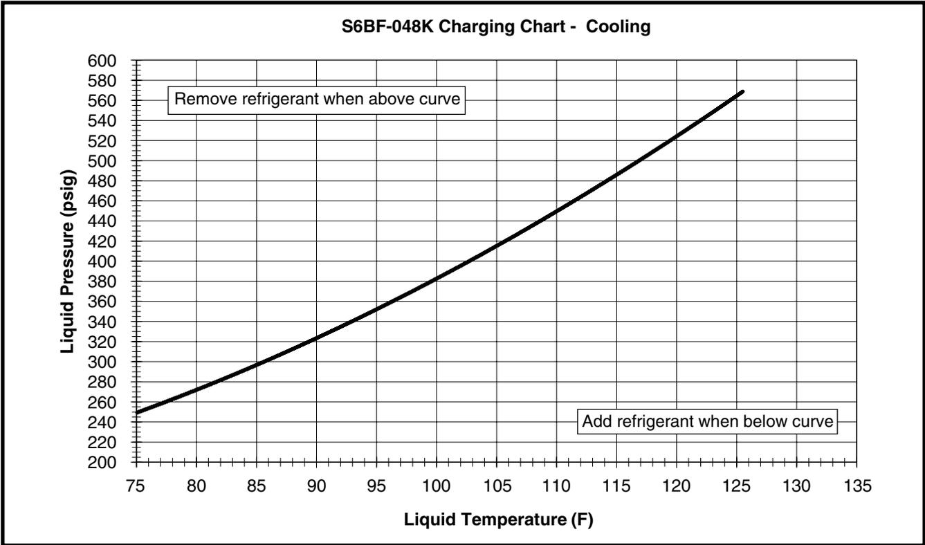
**Figure 6. Charging Chart for 4 Ton Units
