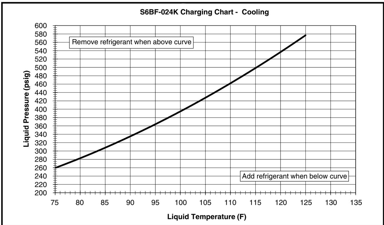
**Figure 2. Charging Chart for 2 Ton Units
