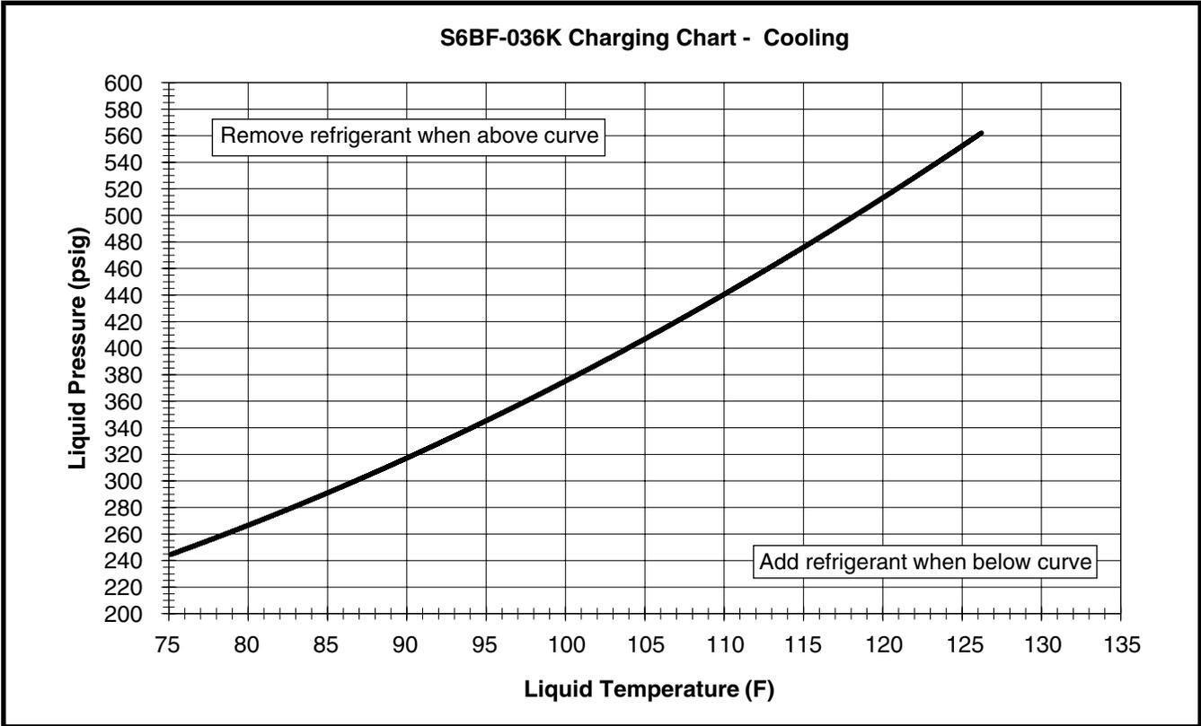
**Figure 4. Charging Chart for 3 Ton Units
