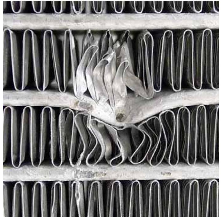
Figure 3. Damaged Micro-Channel Example
