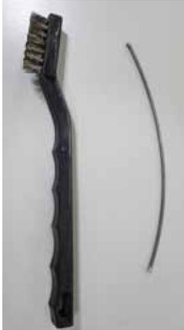
Figure 1. Steel Brush & Brazing Rod
