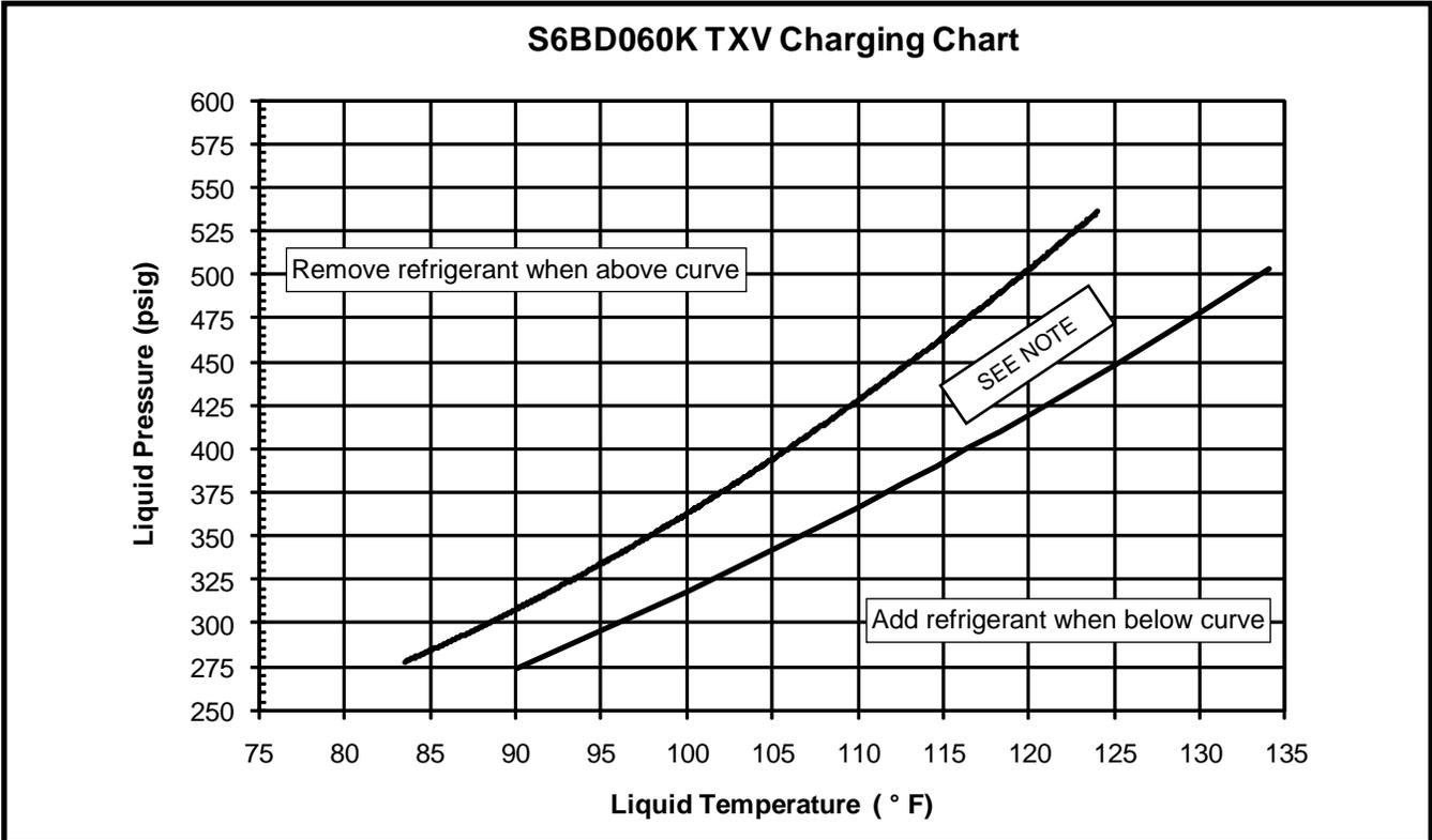
Figure 8. Charging Chart for 5 Ton Units - TXV Matches
