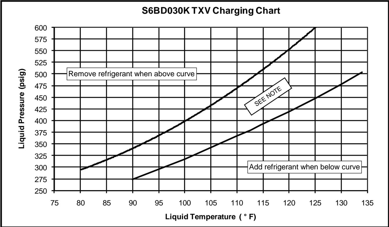
Figure 4. Charging Chart for 2.5 Ton Units - TXV Matches
