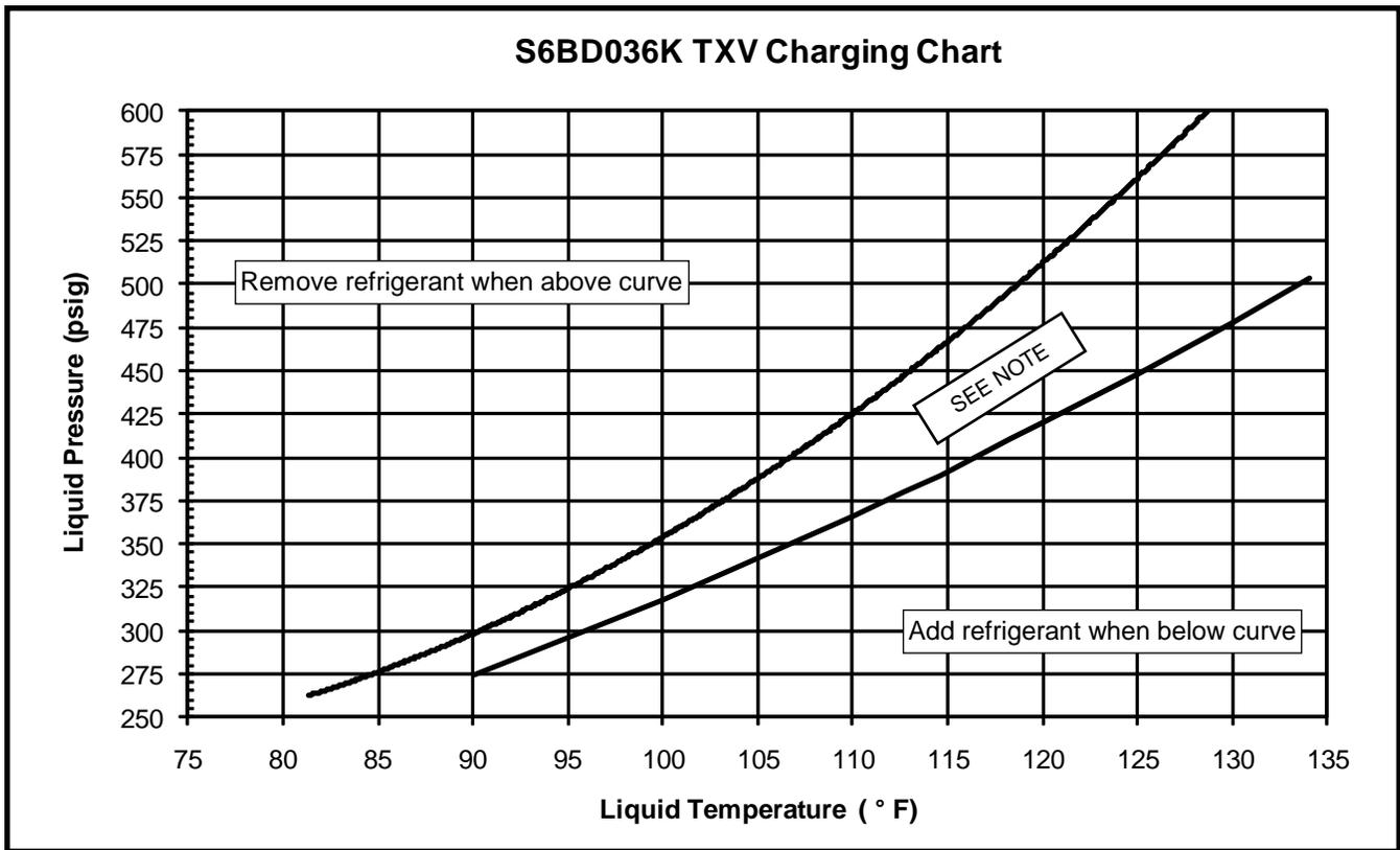
Figure 5. Charging Chart for 3 Ton Units - TXV Matches
