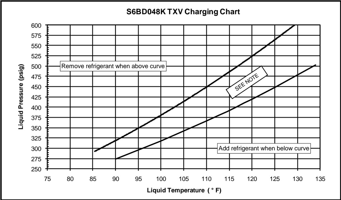
Figure 7. Charging Chart for 4 Ton Units - TXV Matches
