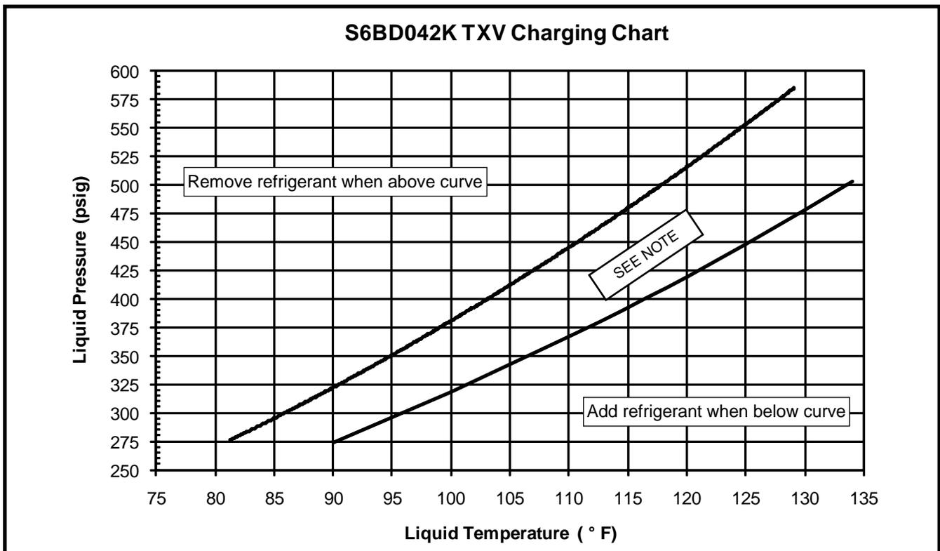
Figure 6. Charging Chart for 3.5 Ton Units - TXV Matches
