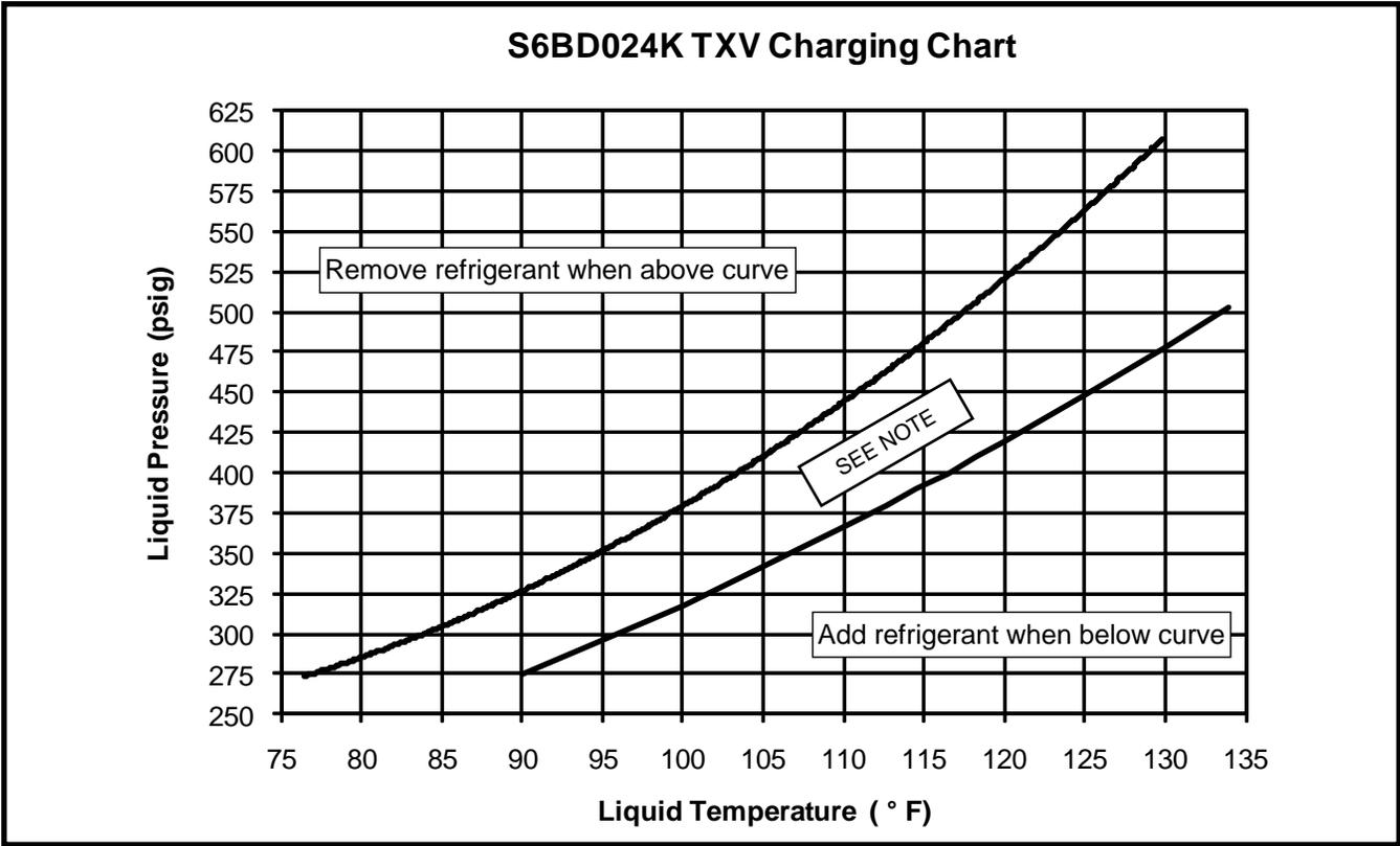
Figure 3. Charging Chart for 2 Ton Units - TXV Matches
