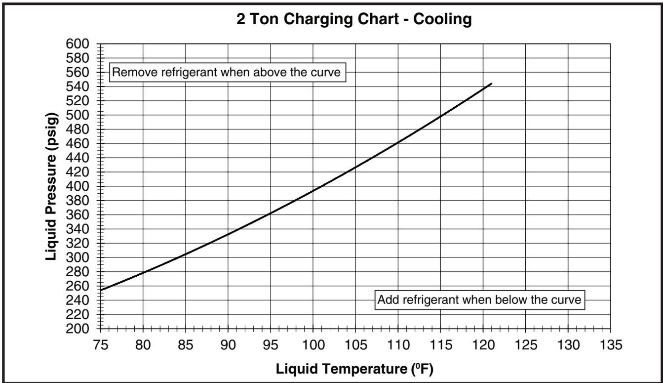
**Figure 7. Charging Chart for 2 Ton Models
