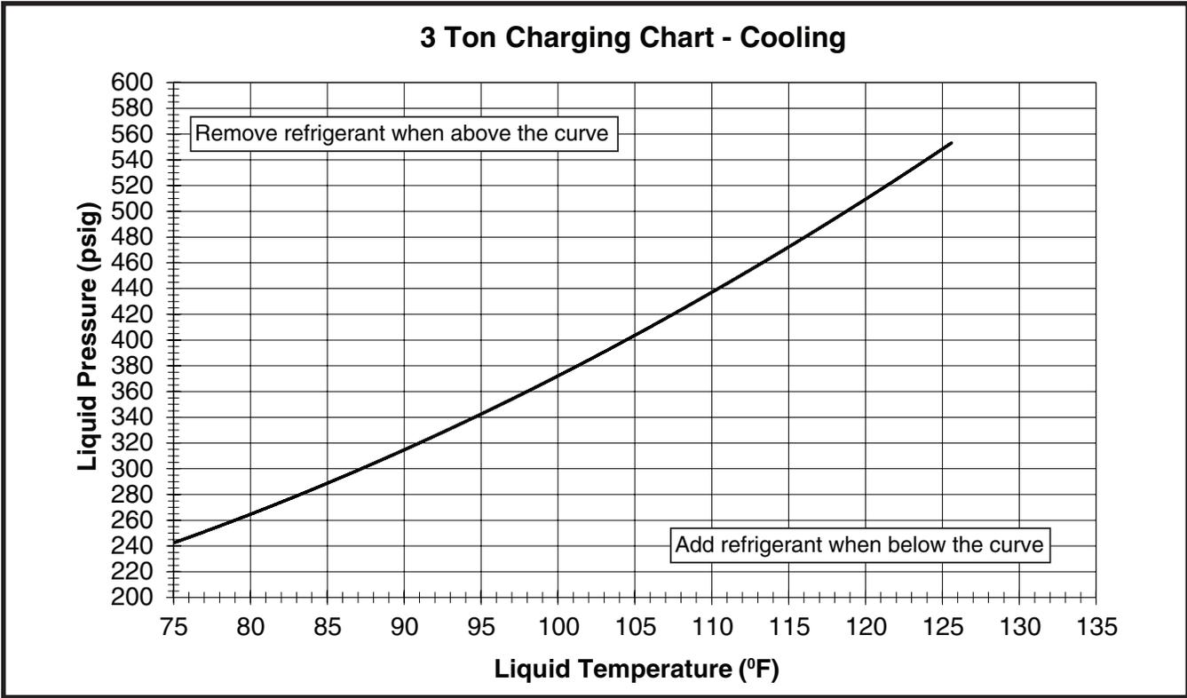
Figure 9. Charging Chart for 3 Ton Models
