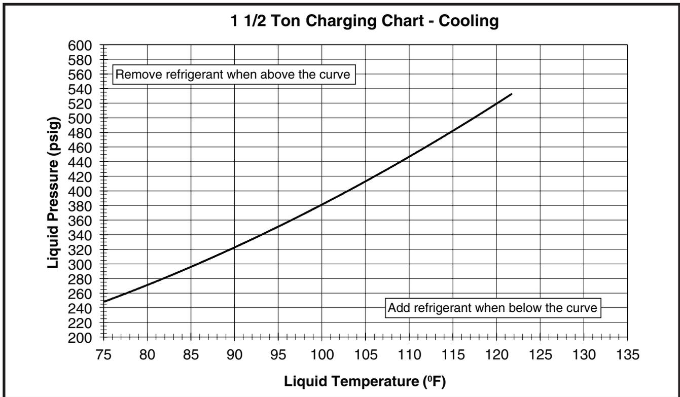
Figure 6. Charging Chart for 1.5 Ton Models
