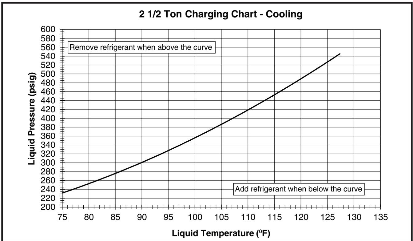
**Figure 8. Charging Chart for 2.5 Ton Models
