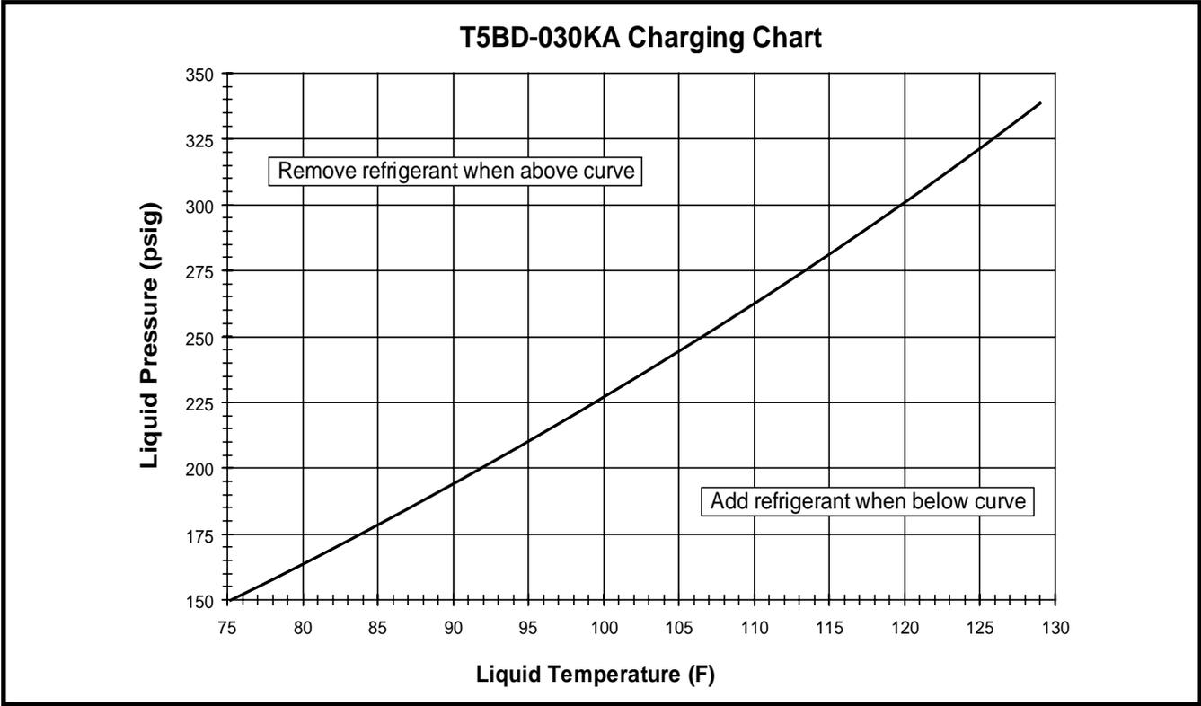
**Figure 7. Charging Chart for 2.5 Ton Units**
