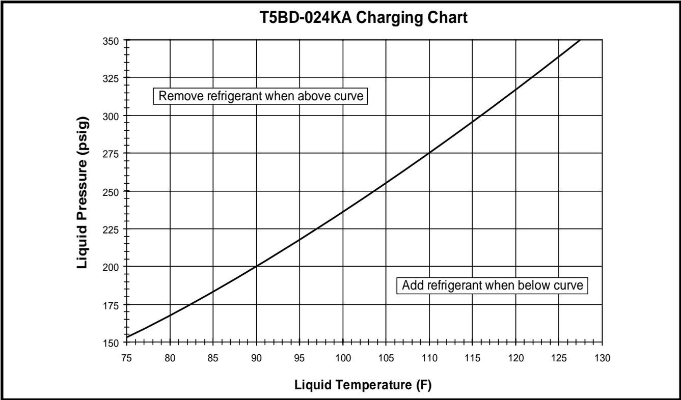
**Figure 6. Charging Chart for 2 Ton Units**
