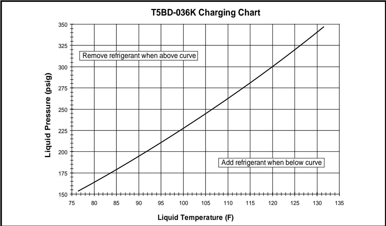
**Figure 8. Charging Chart for 3 Ton Units**
