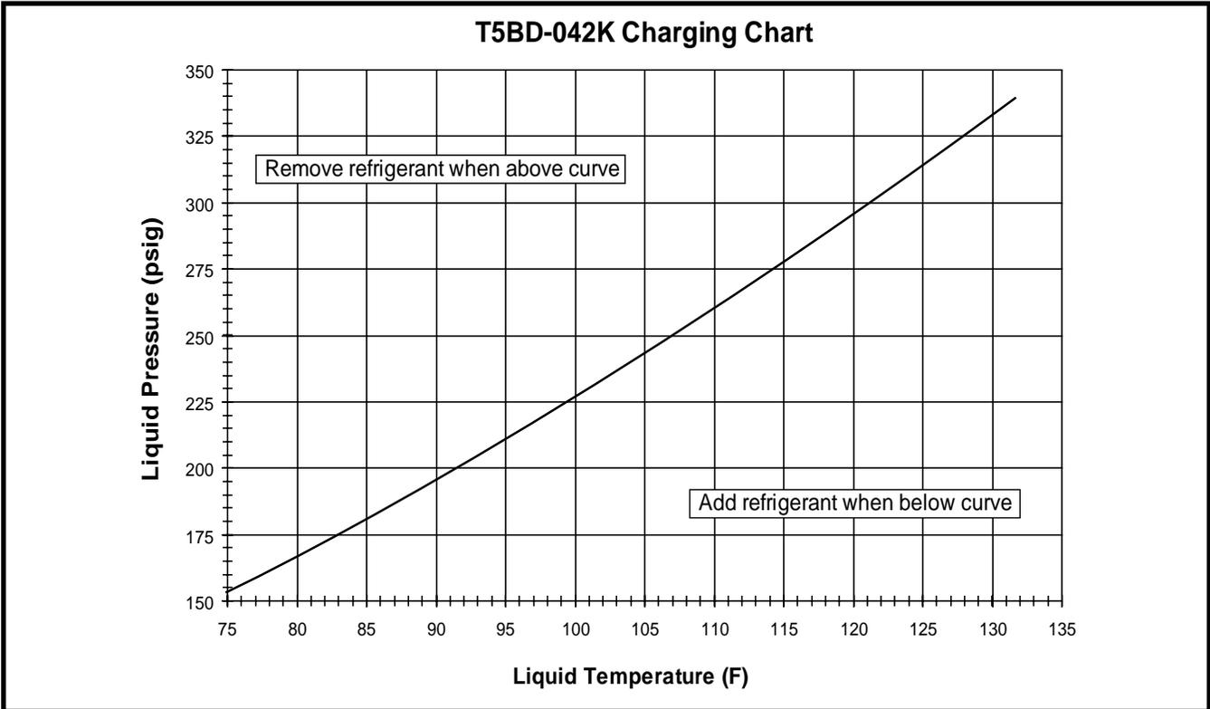
**Figure 9. Charging Chart for 3.5 Ton Units**
