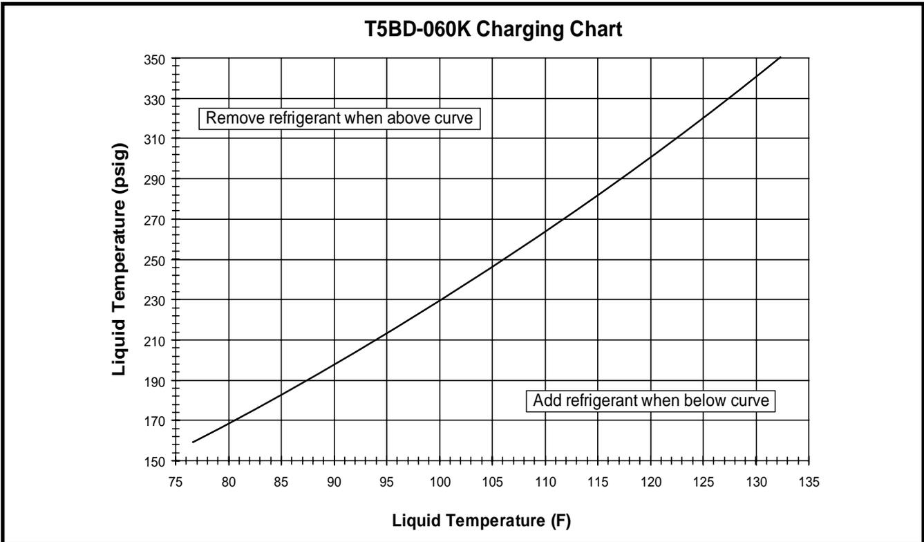
Figure 11. Charging Chart for 5 Ton Units
