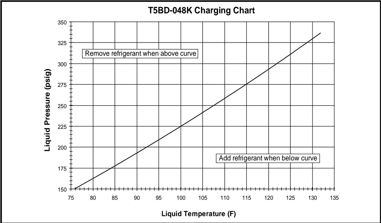
Figure 10. Charging Chart for 4 Ton Units
