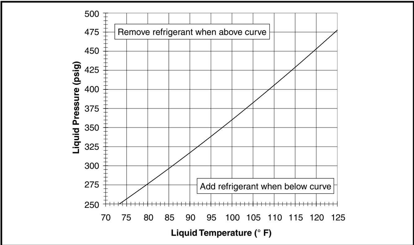
Figure 7. Charging Chart for 5 Ton Units
