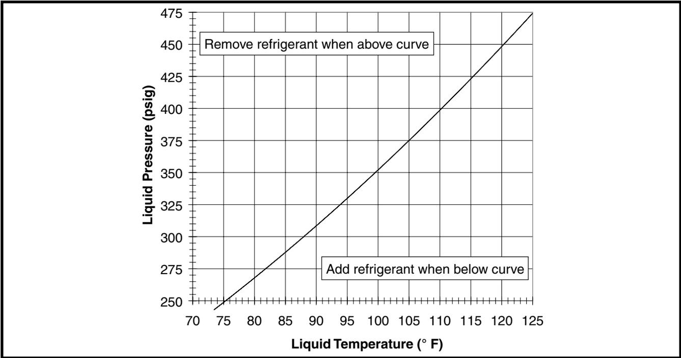
Figure 4. Charging Chart for 2 Ton Units
