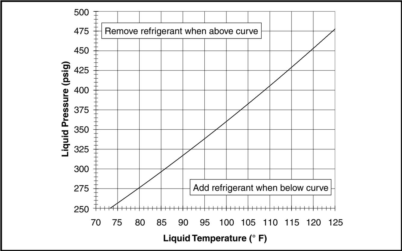
Figure 6. Charging Chart for 4 Ton Units
