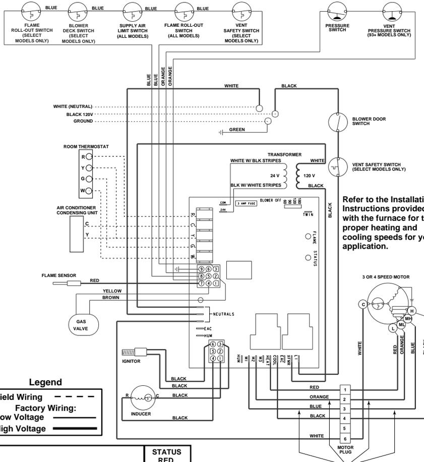
Refer to the Installation Instructions provided with the furnace for the proper heating and cooling speeds for your application.
