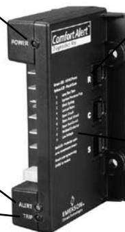
Pass Through Ports Detect Run/Start Current; Spade Connectors Detect Tstat Demand and Pilot Voltage; Microprocessor Monitors Behavior To Determine Faults
