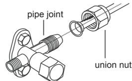
4. Tighten the union nut with torque wrench by referring to the sheet below.
