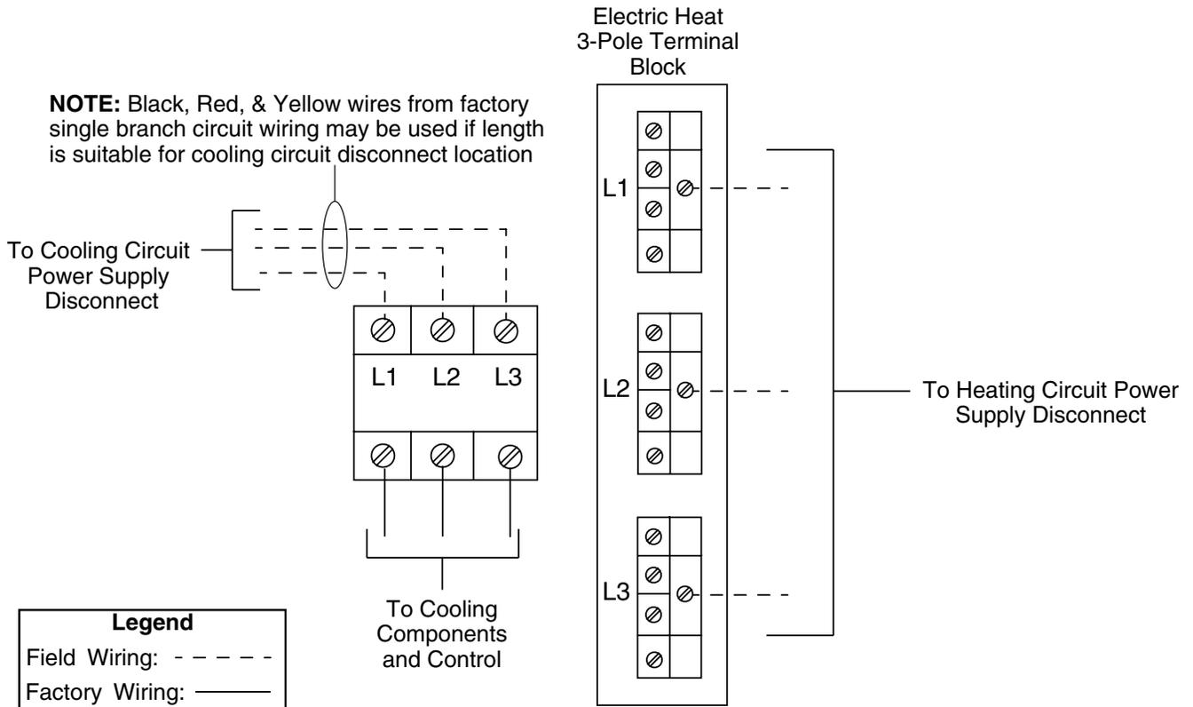
Figure 13. Single and Dual Power Supply Connections
