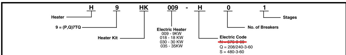
Figure 1. Heater Kit Identification Code
