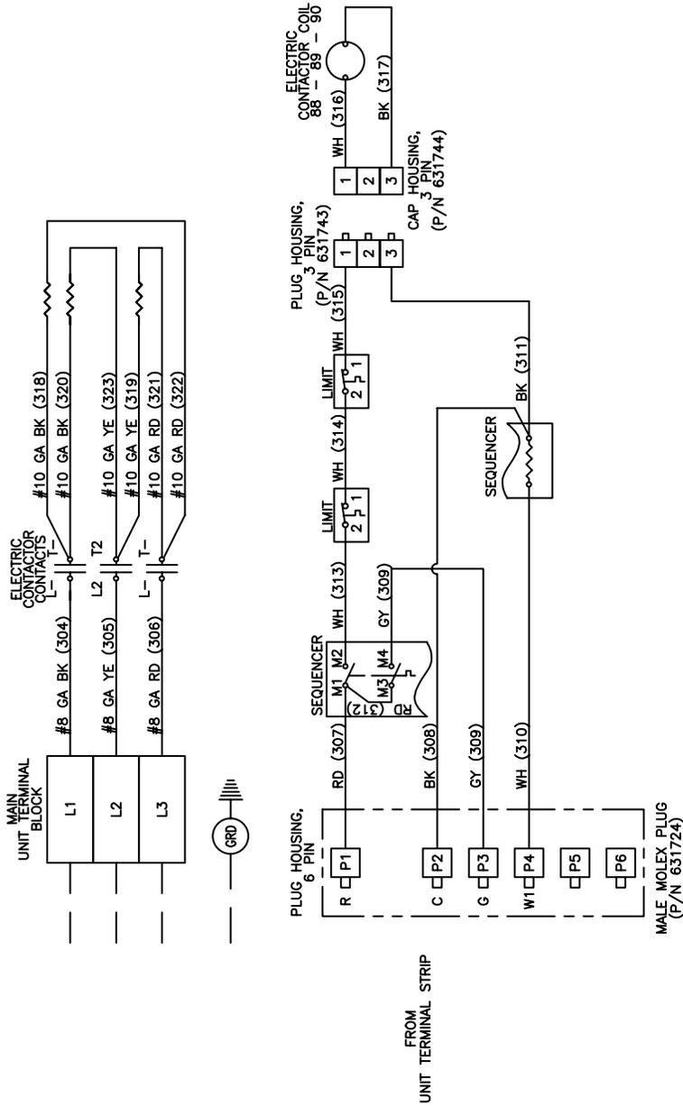
Figure 14. Wiring Diagram for 9 kW, 240V, 3-Phase
